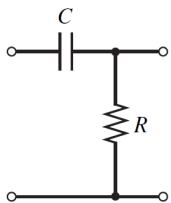
a. Plot  $|H(f)|$  and find and mark the 3dB cutoff =  $f_{3dB}$ .
